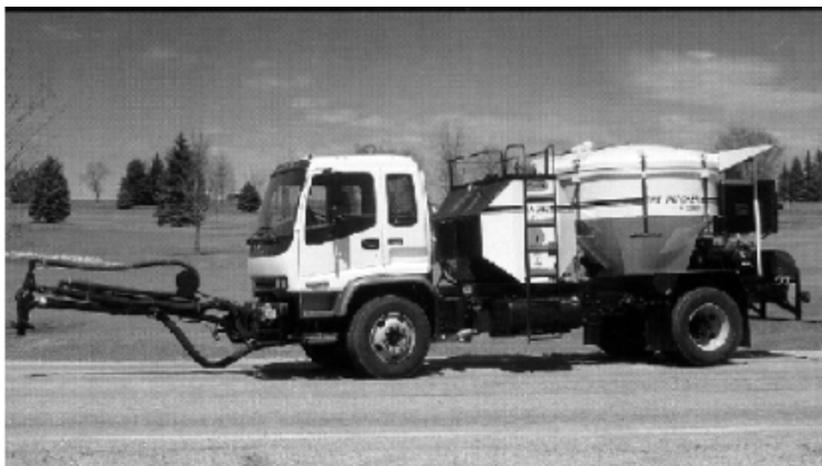
**Figure 2. RA-300 Spray Injection Patcher**
